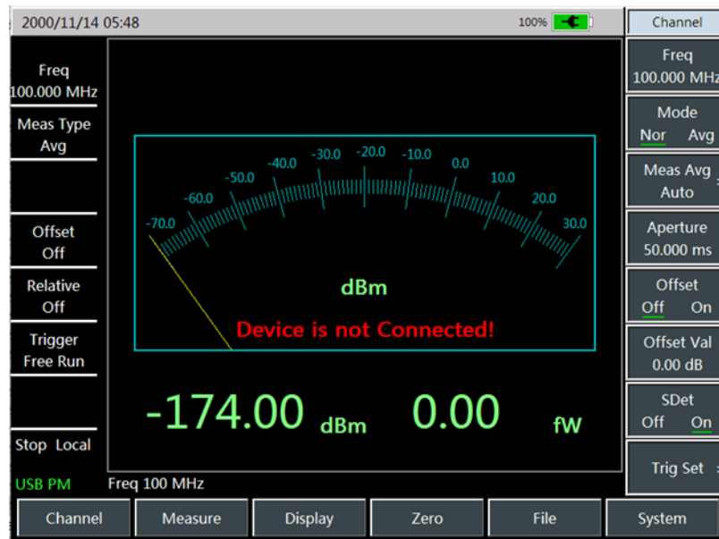
Figure 8-2 USB Power Measurement Interface
