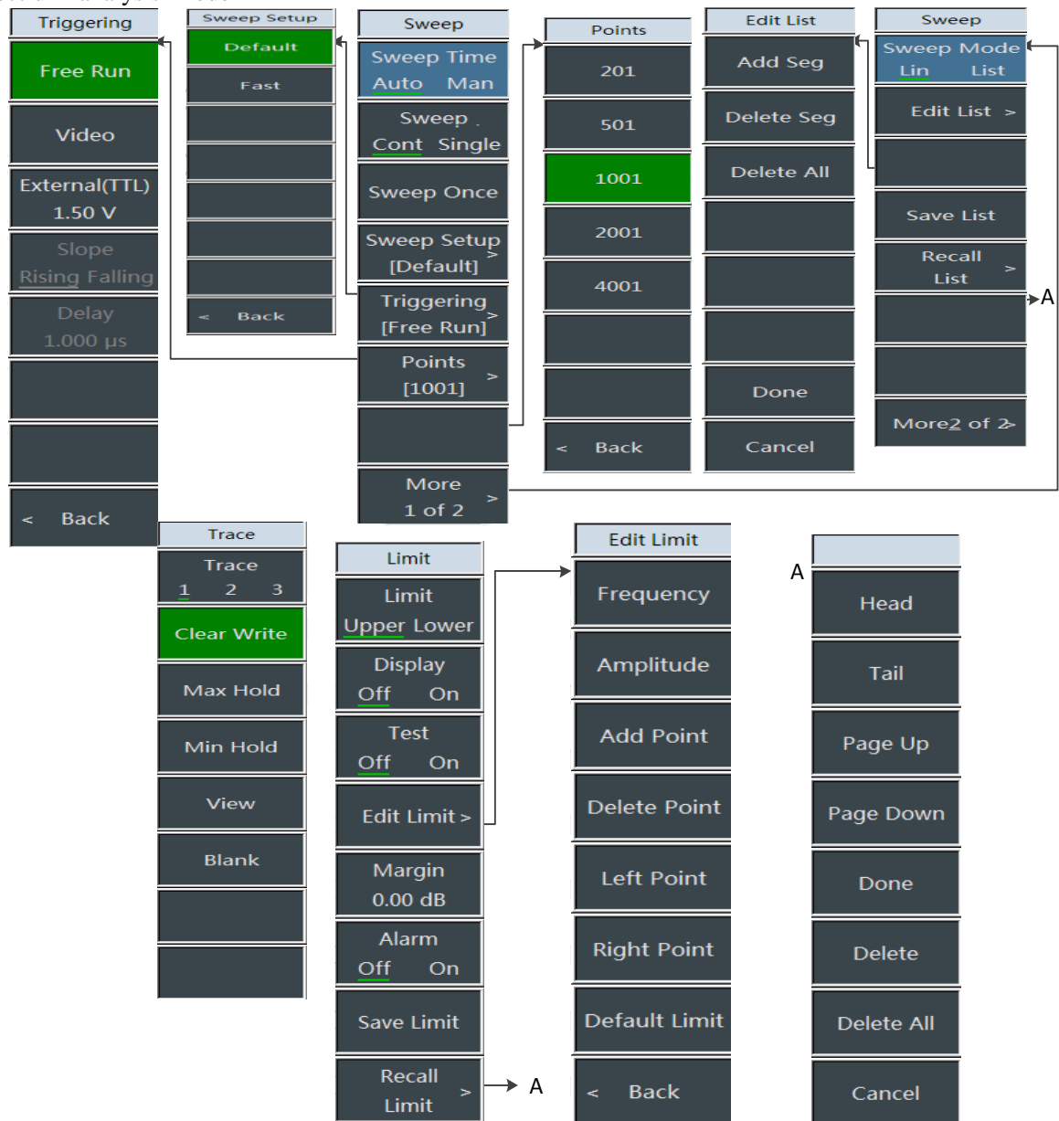
Figure 5-29 Structure of Sweep, Trace and Limit Menu
