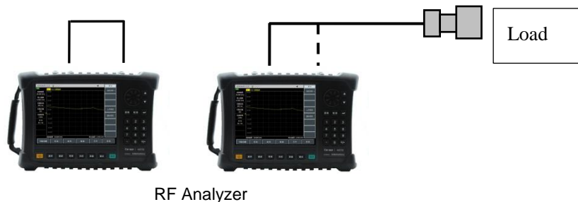
Figure 16-6 Block Diagram of Dynamic Range and Transmission Tracking Test
