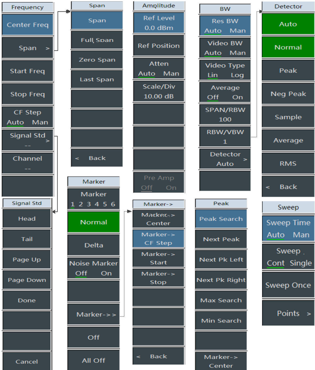
Figure 9-4 Overall Menu Block Diagram of Interference Analysis
