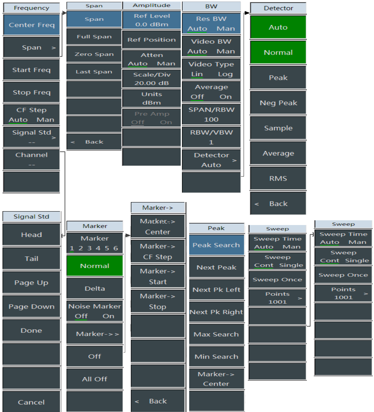
Figure 14-5 Overall Menu Block Diagram of Signal Analysis
