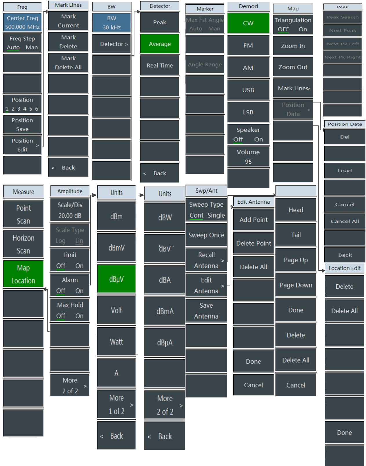
Figure 12-5 Overall Menu Block Diagram of Location analyzer
