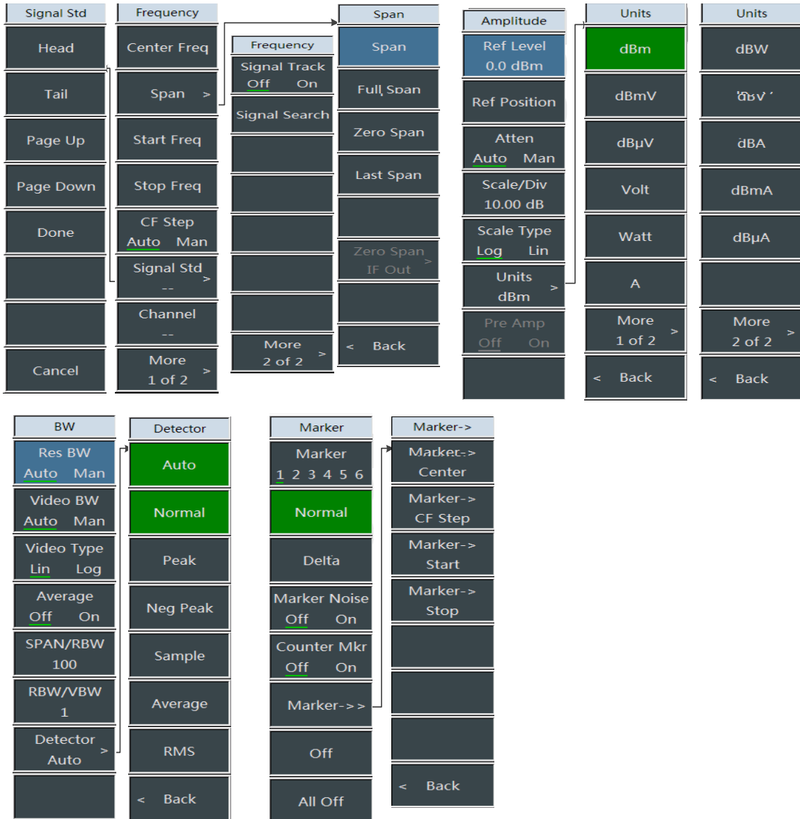
Figure 5-28 Structure of Frequency, Amplitude, Bandwidth and Marker Menu
