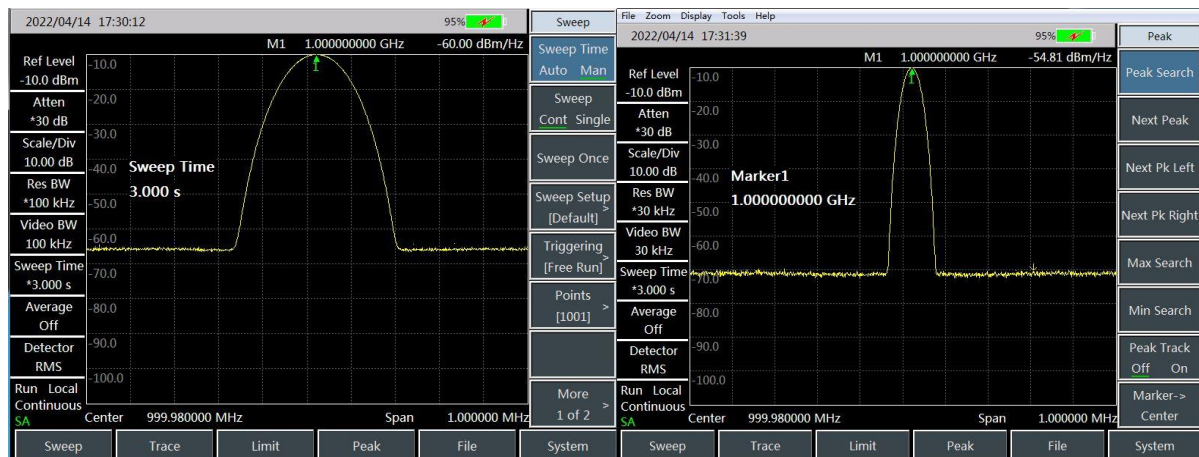
Figure 5-11 Measure Noise with Noise Marker Function
