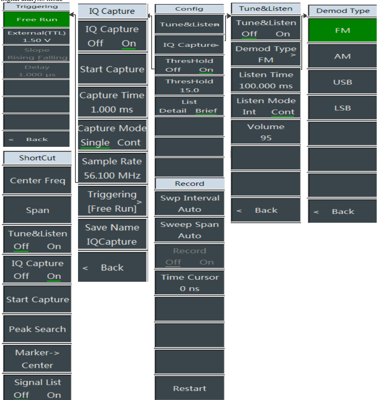
Figure 14-6 Overall Menu Block Diagram of Signal Analysis (Continued)
